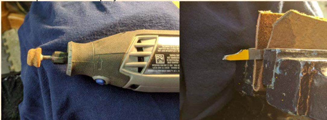
Picture 8. On the left, the Dremel tool with grinding bit attached. On the right, the graver tang after the excess material has been removed.
