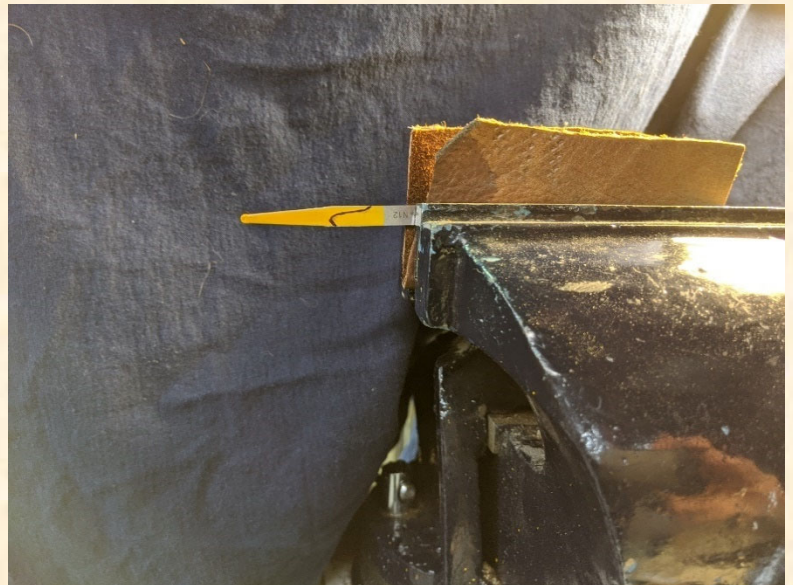
Picture 5. Graver, wrapped in leather, mounted in the vise for cutting and grinding the tang.
